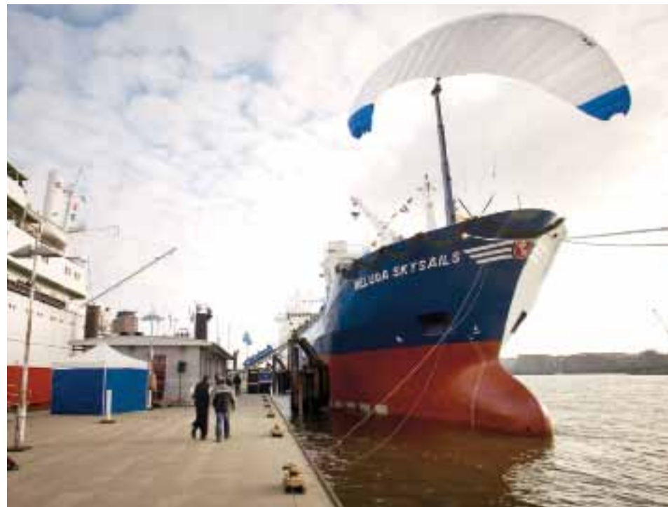
Below: cargo vessel Beluga SkySails about to embark on her maiden voyage equipped with an auxiliary towing kite. British naval architect Rob Humphreys is working on yacht concepts that incorporate the same technology.
