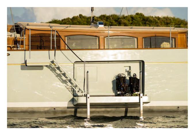
To facilitate the loading / unloading of scuba dive tanks, there is a Lloyd's certified hatch recessed into the hull that is accessible from the side bathing platform. The platform and dockside access are both served by a portable, lightweight carbon composite boarding ladder to the main deck.
