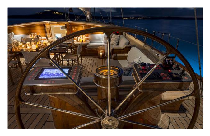
Moreover, Elfje is the first superyacht known to have as her primary steering, approved by Lloyd's, a complete mechanical system free of electric circuitry: physical mechanics at their finest. Working together with Class and Edson Marine, the shipyard developed a practical and sophisticated engineering approach that ensures a balanced and 'true' feel to the helm providing a system that manages human power to accomplish the controlling of force and movement.
