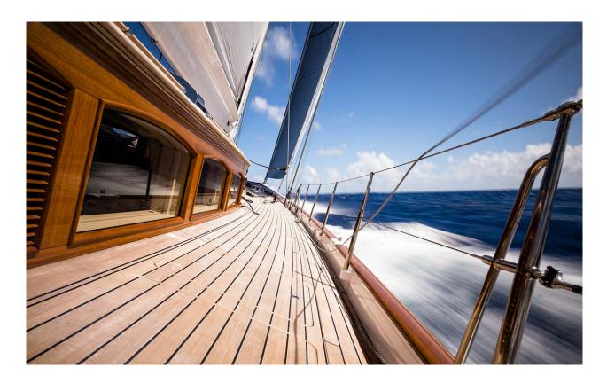
On deck, an expanse of teak decking flows from fore to aft with borderless, flush deck hatches and under-deck hinges to add a final measure of visual simplicity. Further evidence of attentive execution can be seen with the zero maintenance practicality of electro-polished stainless steel hatch gutters and custom designed steering consoles in teak-veneered carbon composite.
