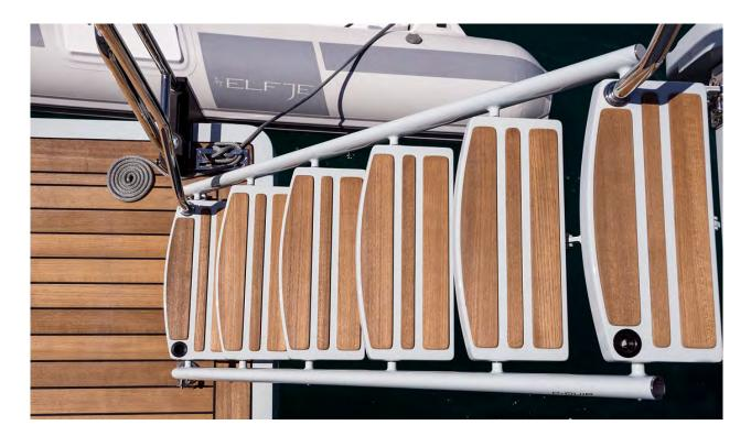
The platform and dockside access are both served by a portable, lightweight boarding ladder to the main deck.
