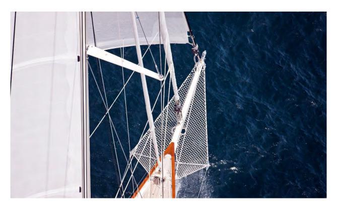
A snubbing line is run out to the bow for longer periods at anchor which, it should also be noted, can be fully deployed manually in the event of an emergency.
