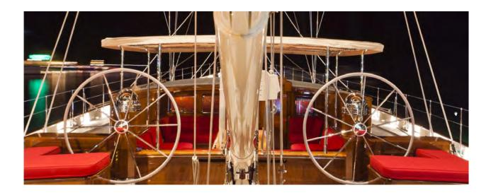
Twin helms make obvious seafaring sense when campaigning a yacht of this size and power. Their positioning is designed to optimise sightlines both to sails and to the external environment, while the more contemporary visual note they introduce has been carefully nuanced through traditional styling and the use of stow-away displays and controls.
