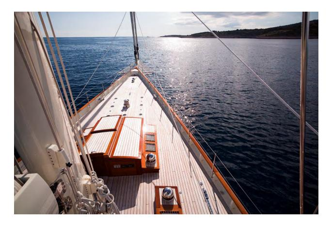
The clean parallel to centre line-planked decks are surmounted by teak-clad pilot houses and complemented by other sympathetic period features such as skylights with bevelled glass and polished stainless steel mushroom air vents.
