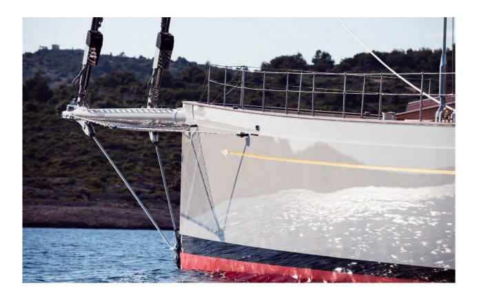
With her plumb bow, long waterline, low wetted-surface areas and high sail area to displacement ratio, Kamaxitha is designed to deliver fast acceleration and high speeds.
