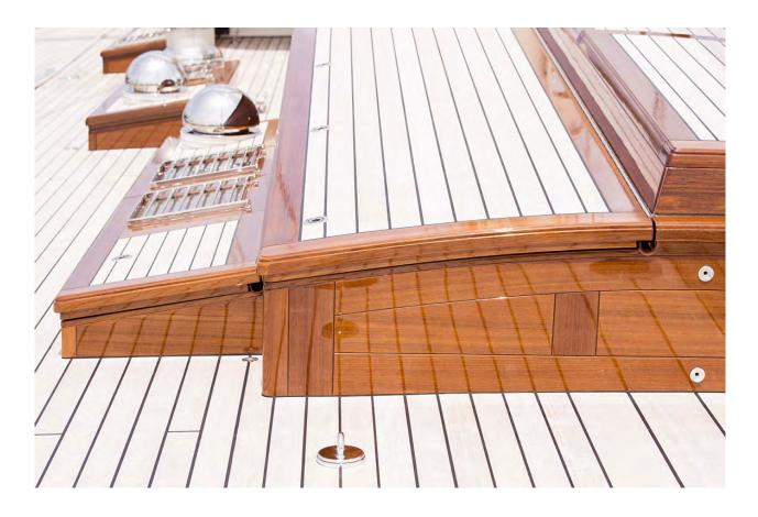
Sympathetic period features include two beautifully-joinered skylights inset with bevelled glass. In keeping with tradition, deck planks are laid fore-andaft parallel to the yacht's centreline, running without interruption, it seems, through hatches that show no visible margin planks.
