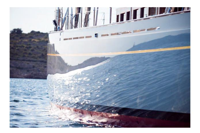
With no portholes to interrupt her topsides Kamaxitha looks both traditional and purposeful. Her fine hull lines, accentuated by a gold-leafed cove stripe and visually uninterrupted teak cap rail, are complemented by a traditional 'open bulwark', clean open deck spaces and neatly proportioned teak-clad deckhouses.
