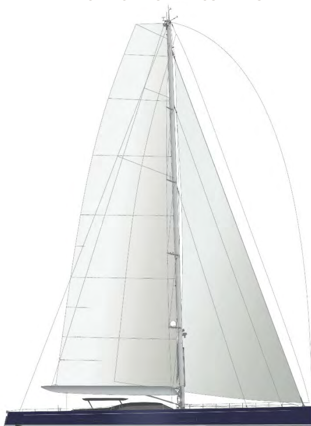
CARBON RIG WITH CURVED SPREADERS
