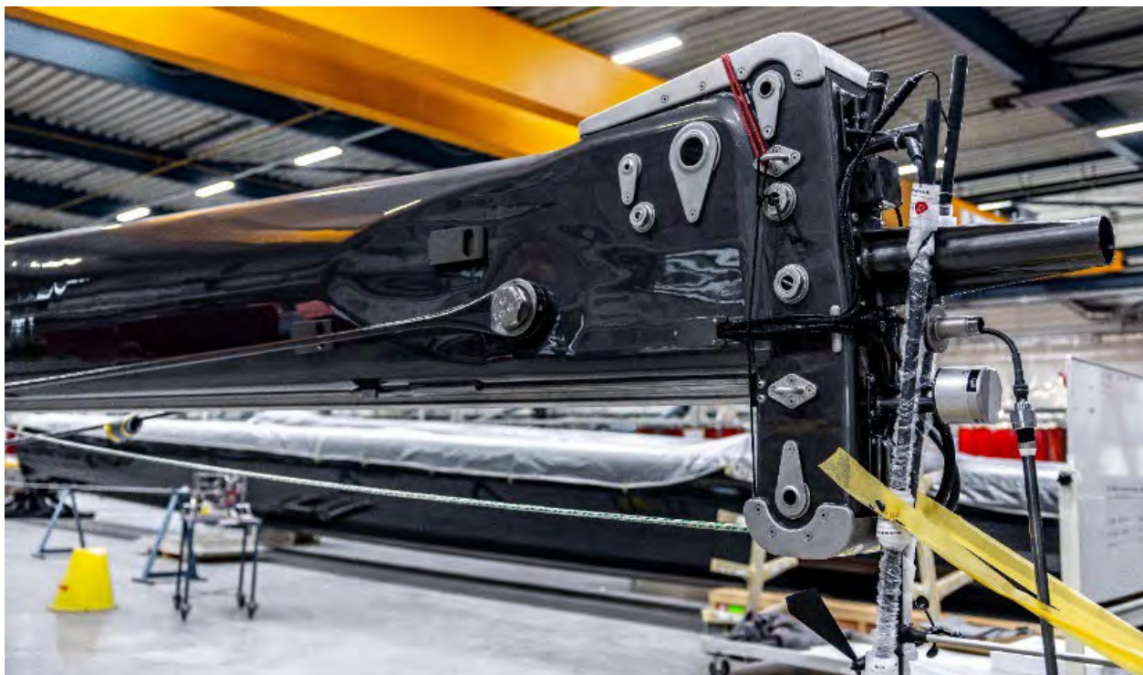
ABOVE: NILAYA'S MAST IS TAPERED IN TWO DIRECTIONS AT THE TOP
