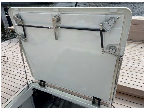
BELOW: CARBON LAZARETTE HATCH WITH MANUAL CENTRAL LOCKING SYSTEM (NOTE THE INTERCONNECTING CARBON BARS) AND HYBRID CARBON / ALUMINUM CAPTIVE WINCHES
