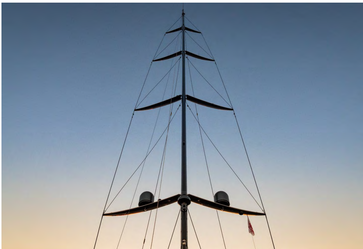
CARBON RIG WITH CURVED SPREADERS
