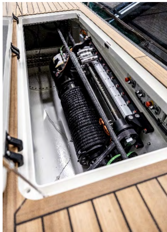
BELOW: CARBON LAZARETTE HATCH WITH MANUAL CENTRAL LOCKING SYSTEM (NOTE THE INTERCONNECTING CARBON BARS) AND HYBRID CARBON / ALUMINUM CAPTIVE WINCHES
