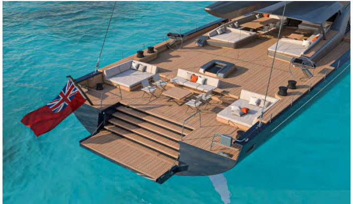
RENDERING (ABOVE) AND REALITY (BELOW). THE GRAND STAIRCASE CAN BE RAISED FOR LAUNCHING THE CREW TENDER
