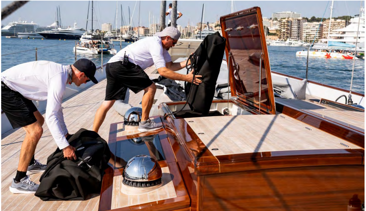
BESPOKE COWL VENTS AVOID SNAGGING OF SHEETS ON THE FOREDECK
