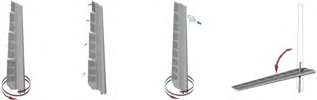
WING SAIL FROM LEFT TO RIGHT: UNSTAYED AND INFINITE ROTATION; INDIVIDUAL FLAP CONTROL TO MANAGE TWIST AND POWER; FEATHERING WHEN STATIONARY; TILTABLE FOR PASSING BRIDGES, RARE EXTREME WEATHER CONDITIONS AND YARD PERIODS
