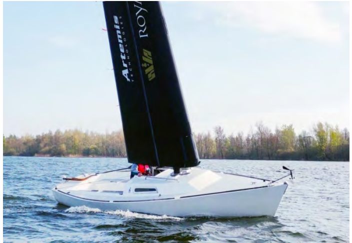
TESTING OF THE WING SAIL DEVELOPED BY RONDAL IN COLLABORATION WITH ARTEMIS TECHNOLOGIES
