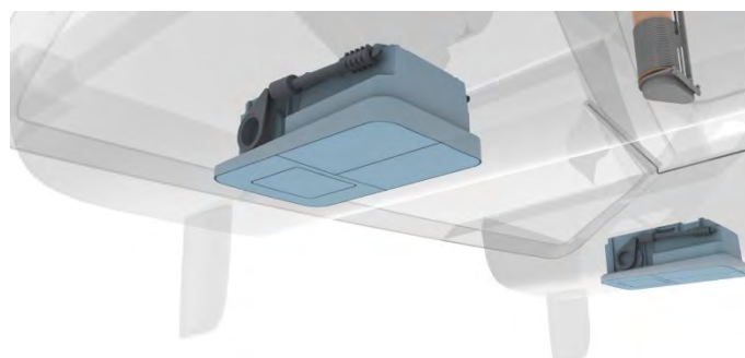
AERA'S ELECTRIC PROPULSION SYSTEM (AND SARISSA'S IN CENTER): FORWARD-FACING AND RETRACTED (BOTTOM)
