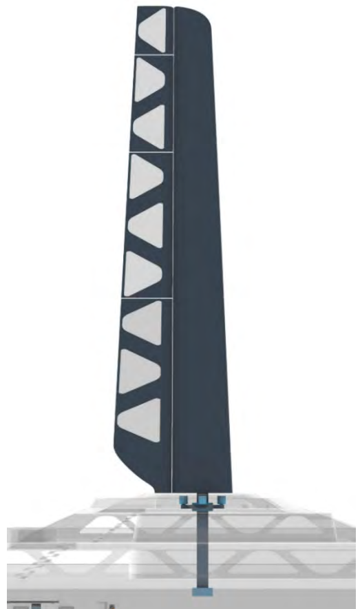
AERA'S WING SAIL RESTS ON TWO BEARINGS INSIDE THE YACHT
