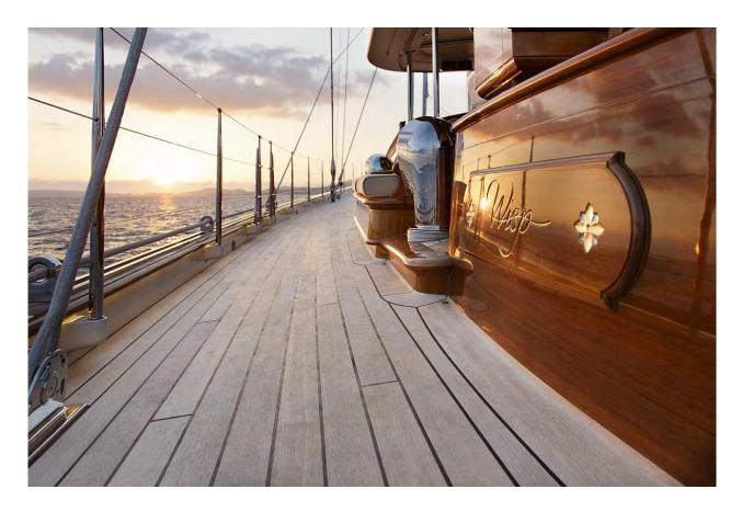
Wisp features traditional waterfall margins between the teak decking and the superstructures – a detail requiring much thicker pieces of carefully selected timber to provide a consistent grain and perfect fit and finish.
